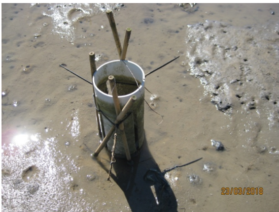
Figure 4. Tube design used after 2018. Tubes were inserted only 25 mm below the sediment, and secured by 700 mm bamboo stakes and cable ties.
