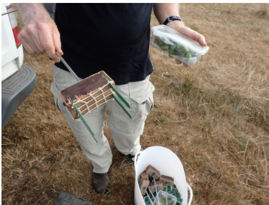
Figure 8. Mangrove seed held in place by double layer of 9 mm meat netting inside a slotted PVC tube (upper). Device used to insert builders spacers and a single layer of 15 mm meat netting to hold seeds in place (lower).
